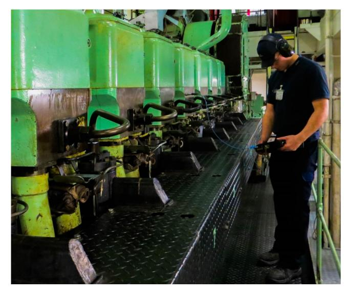
Vibration monitoring of Marine Diesel Engine
