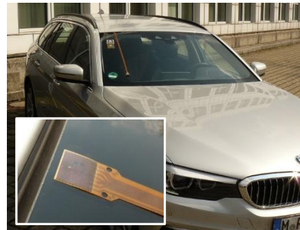
EMFT: sensors on curved surfaces
